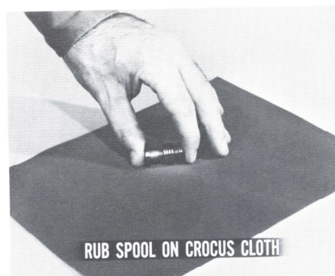
Fig. 26—Do not round off valve spool lands
