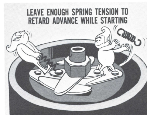
Fig. 13—Remove heavy spring and stretch the other
