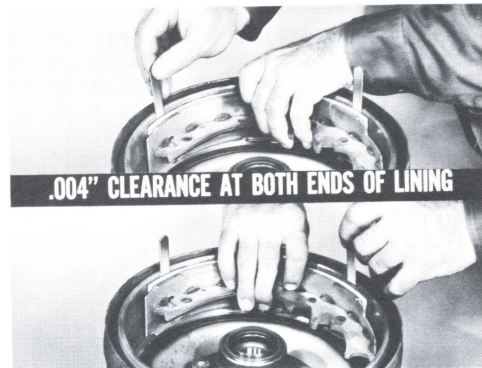
Fig. 12—Lining radius must be correct
