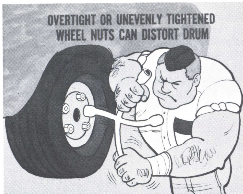
Fig. 6—Don't tighten nuts too much
