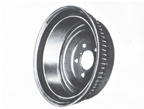
Fig. 27—Ribbed and flared rear brake drum
