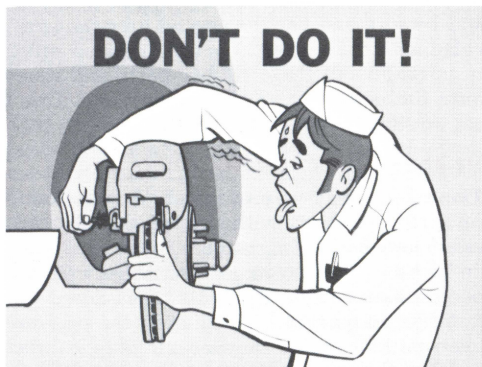
Fig. 35—Install the bushings in the caliper first
